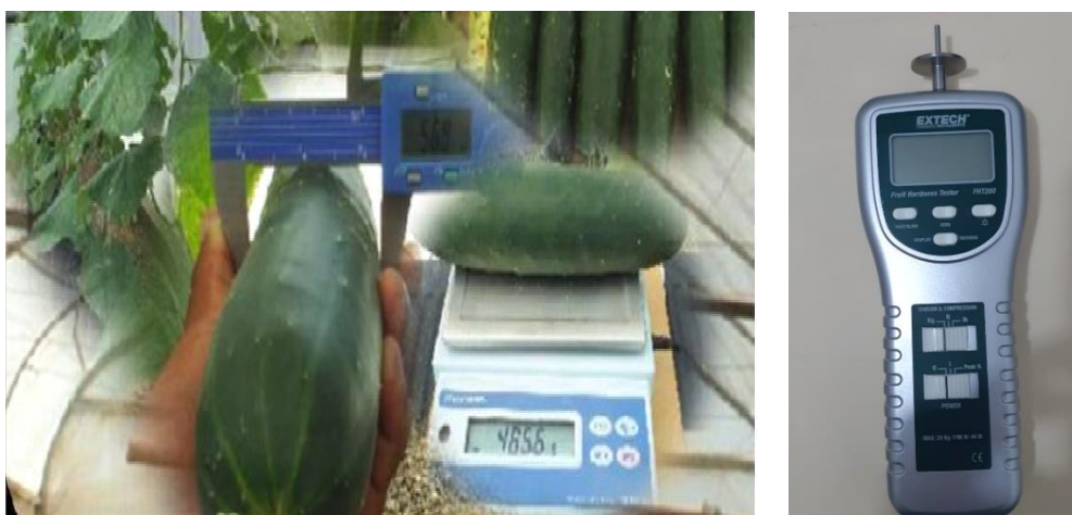
Figure 2. Lab caliper and precision weighing balance (left); Extech penetrometer (FHT200) (right).
